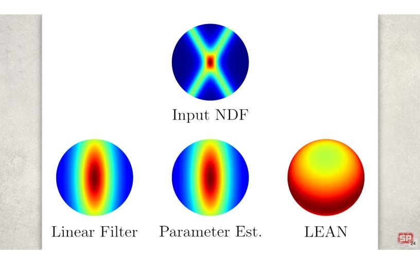
In this case, the input NDF normals are still at 45 degrees from the Z axis, but they are anisotropic "fiber-like" distributions with  $alpha_t = 1$  ( $alpha_b = 0.2$  as before). Note that the input NDF exhibits symmetry around the Z axis, which is captured by both linear filtering and parameter estimation, but not by LEAN.
