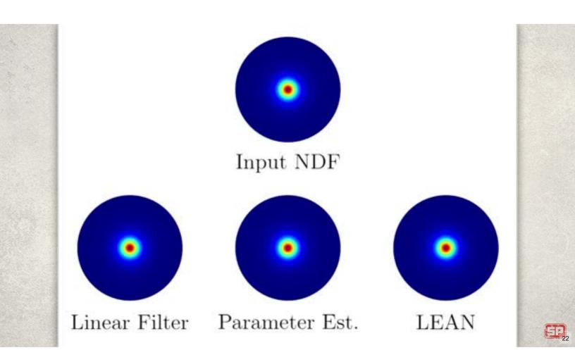
This animation shows an input NDF that is a mixture of two SGGX NDFs, with the three different filtering methods on the bottom. Linear filtering and Parameter Estimation match quite closely in most cases, while LEAN filtering diverges more significantly. The first scenario that I'll point out is here.
