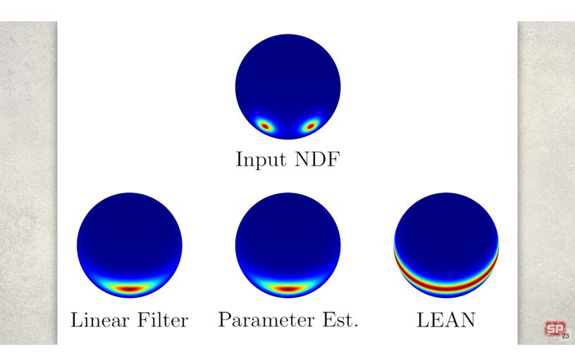
As the input NDF normals deviate from the macro-surface normal (which is the center of the sphere, since we're looking straight down the Z axis), LEAN tends to over-blur compared to the SGGX-based methods. Here the input NDF is made up of two isotropic GGX distributions (alpha\_t = alpha\_b = 0.2) at 45 degree angles from the Z axis.
